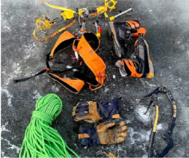
Ice climbers use specialized gear—much of it adapted from or similar to gear used by rock climbers—to scale vertical walls of ice. Typical equipment, clockwise from top, includes: spiked crampons attached to boots; ice screws to anchor ropes; rigid-soled boots; ice axes; a helmet; carabiners to attach to ropes and anchors; insulated gloves; dynamic climbing ropes; and a climbing harness to secure against falls. (Wyoming Truth photo by Ruffin Prevost)
